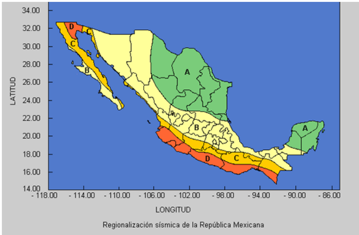
Figure 5.1. Seismic zonation of Mexico according to the 1993 edition of the Manual for Civil Works of the Federal Commission Electricity (MOC-CFE, 1993).
