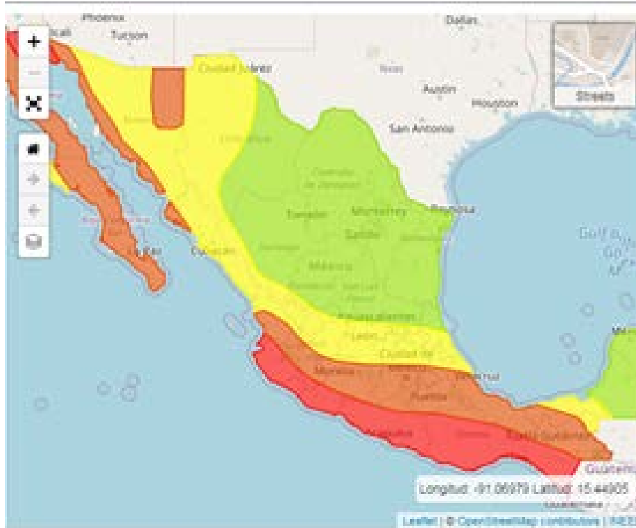
Figure 5.2. Map of iso-acceleration curves to compute the seismic design spectra according to the 2015 edition of the Manual for Civil Works of the Federal Commission Electricity (MOC-CFE) obtained from software platform PRODISIS.
