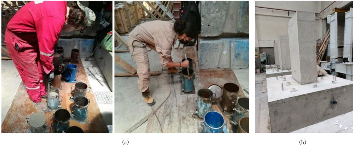
Fig. 3.8—(a) Preparation of cylinders of the foundation and column concrete mix; (b) specimen final state (courtesy: S. M. Alcocer)
