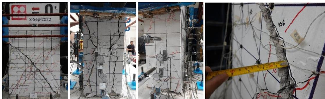
**Fig. 3.41—Damage at a drift of +0.02**
