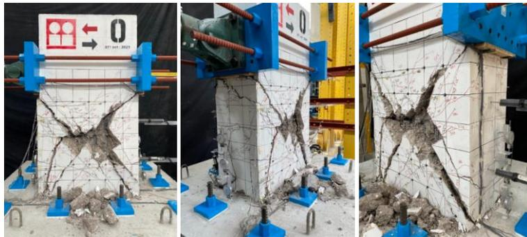
**Fig. 3.29—Column O final state, end of test (courtesy: S. M. Alcocer)**
