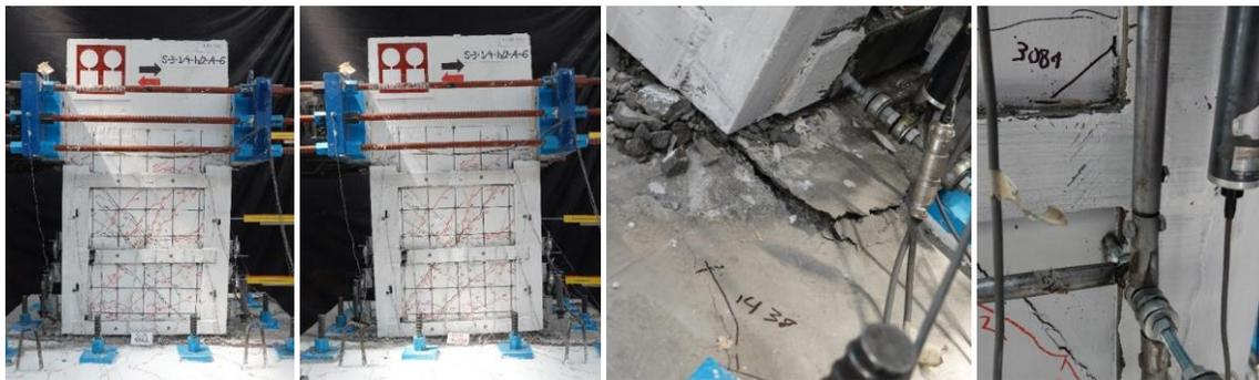
*Fig. 3.86—Damage state at drift of  $\pm 0.04$*
