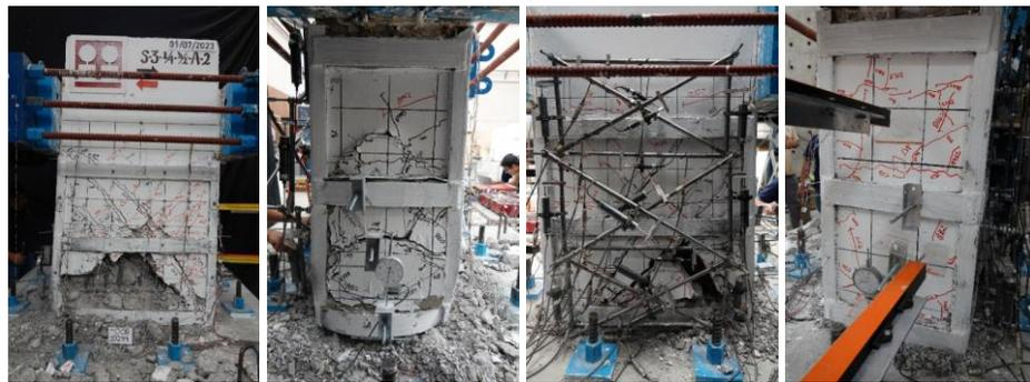
Fig. 3.65—Damage state at a drift of +0.08
