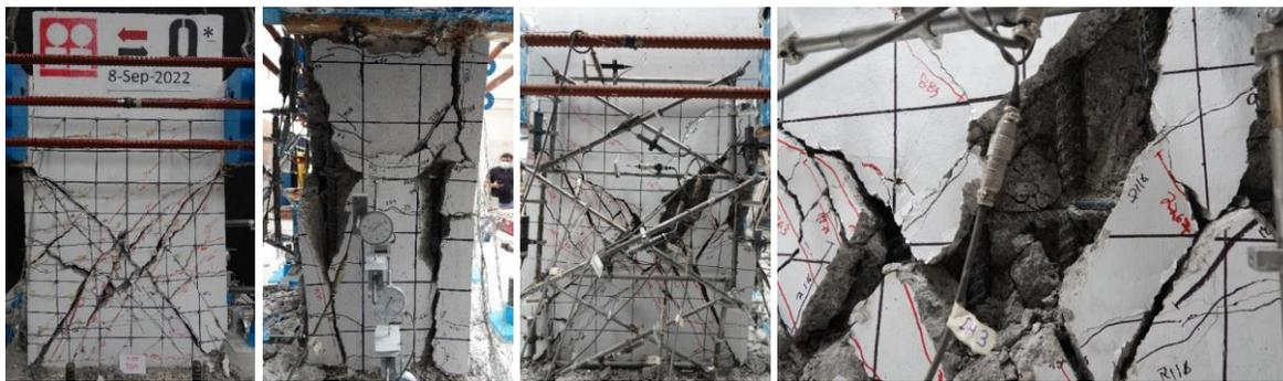
*Fig. 3.44—Damage at a second drift of -0.02*
