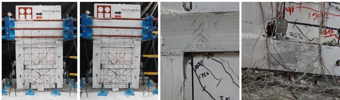
*Fig. 3.88—Damage state at drift of  $\pm 0.055$  when occurred the fracture of a longitudinal bar related to east face*
