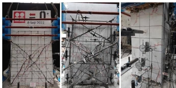
**Fig. 3.42—Damage at a drift of -0.02**
