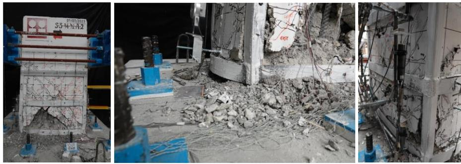
Fig. 3.64—Damage state at a drift of +0.07
