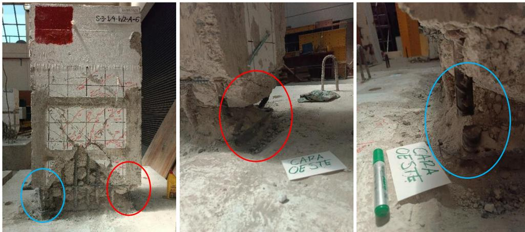
Fig. 3.93—Fracture of longitudinal bars in specimen S9 in west and east face
