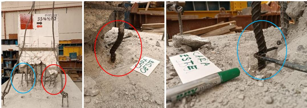
Fig. 3.68—Fracture of longitudinal bars in specimen S8 in east and west face
