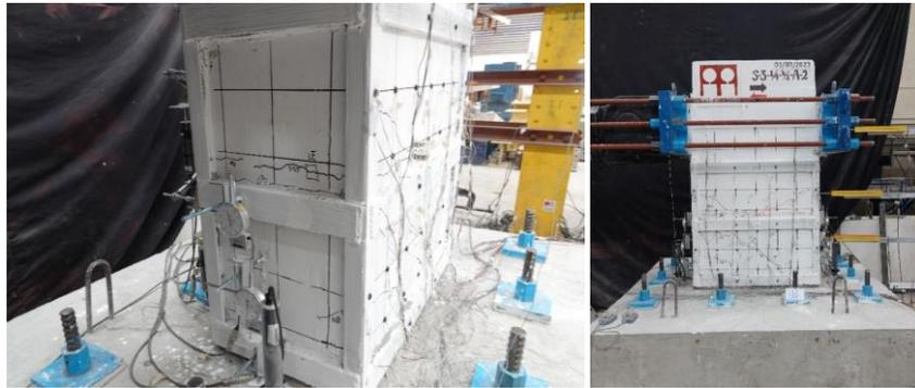
**Fig. 3.55—(a) Transverse crack parallel to steel batten at a drift of +0.0005**
