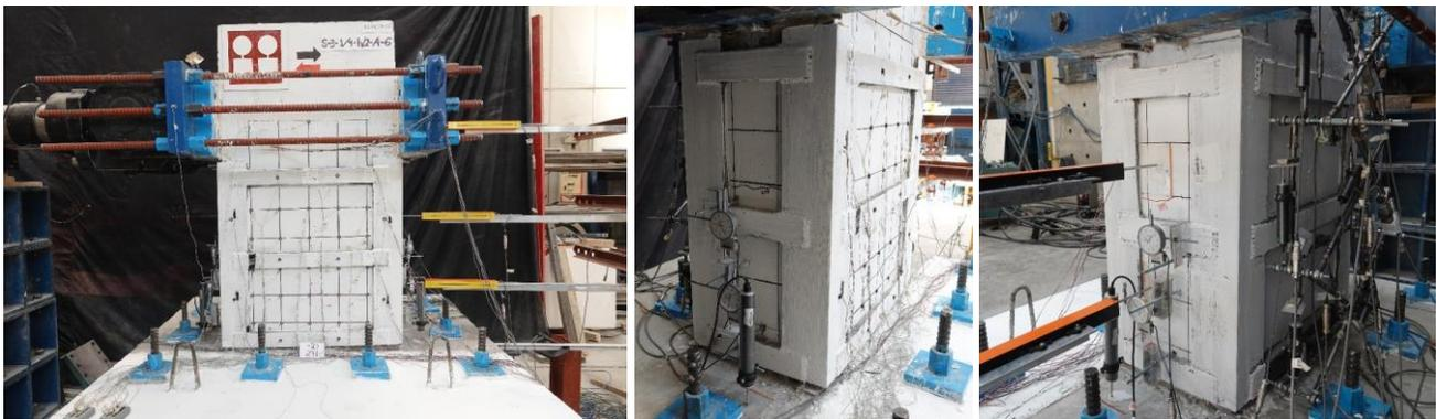
*Fig. 3.79—First horizontal crack at load control of  $\pm 196$  kN*
