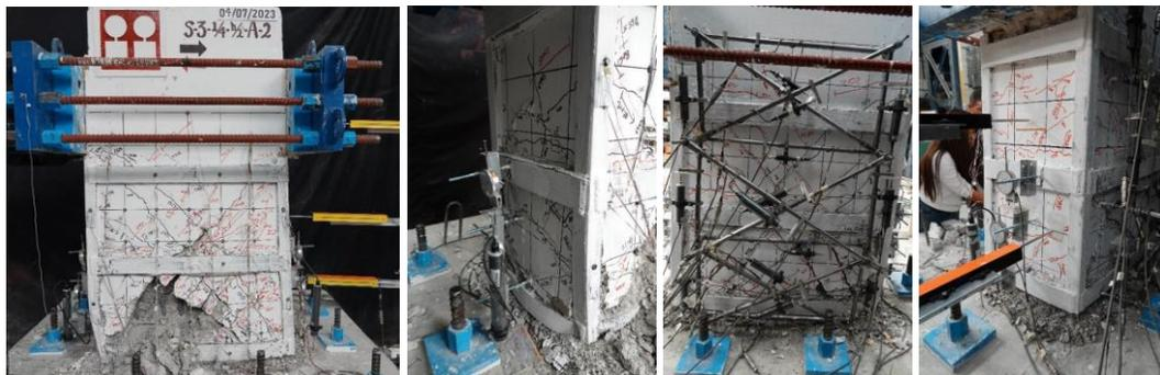
**Fig. 3.63—Damage state at a drift of -0.06**
