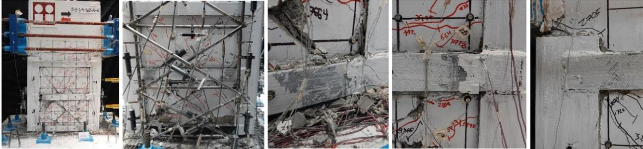
Fig. 3.92—Final damage state of specimen S9
