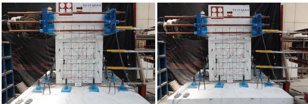
**Fig. 3.83—Damage state at drift of ±0.02**
