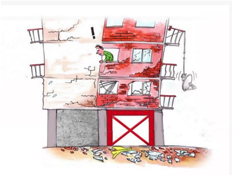
Building with soft first story
